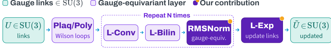
Figure A.1: The L-CNN architecture used with added L-Exp and RMSnorm layers.
