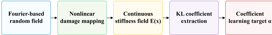
Figure 7: Generation procedure of continuous stiffness fields independent of the KL representation. A continuous spatial variation field is first generated using random Fourier harmonics and subsequently transformed into a damage distribution and Young’s modulus field through nonlinear physical mapping and admissibility constraints. The resulting stiffness field is generated independently, while the underlying spatial variation field is projected onto the KL space afterwards for constructing learning targets.
